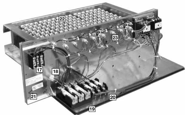
Power hook-up in the field is easy with single-point wiring to a terminal block (**[17]**) and a polarized plug for the low-voltage connection (**[18]**). The electric furnace comes with fuses for the unit (**[19]**) and for the electric furnace (**[20]**), and is UL certified (**[21]**). The electric heating elements are of a wound-wire construction (**[22]**) and isolated with ceramic bushings. The limit switch (**[23]**) protects the design from over-temperature conditions.
