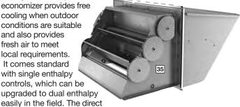
drive actuator combined with gear drive dampers has eliminated the need for linkage adjustment in the field. The economizer control has a minimum position set point, an outdoor-air set point, a mixed-air set point, and a CO2 set point. Barometric relief is standard on all economizers.
