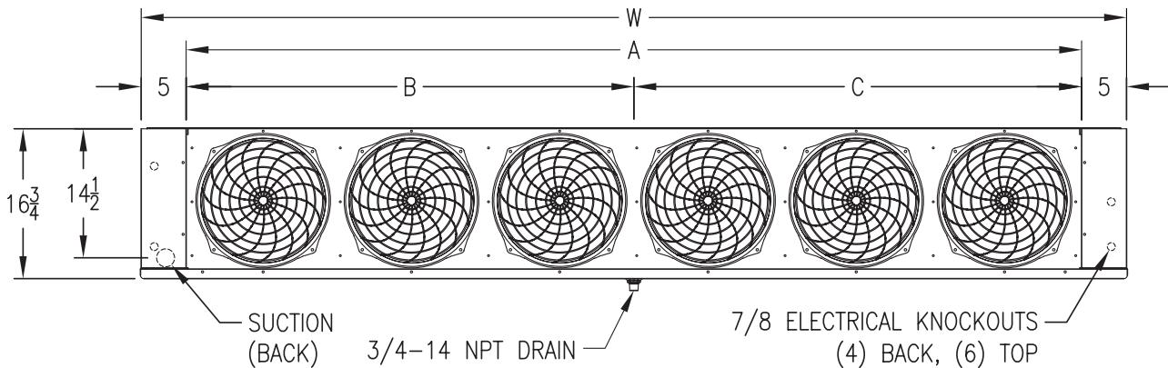
**NOTE:** Refrigerant and electrical connection locations have been changed for the Next-Gen All-Temp design. Standard connections are now opposite of the legacy LP models.
