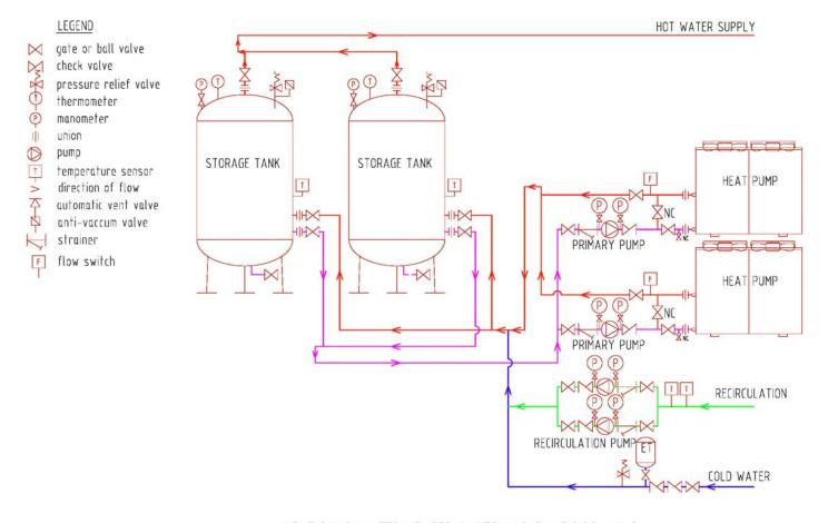
HEAT PUMP WATER HEATER SYSTEM SCHEMATIC DRAWING
