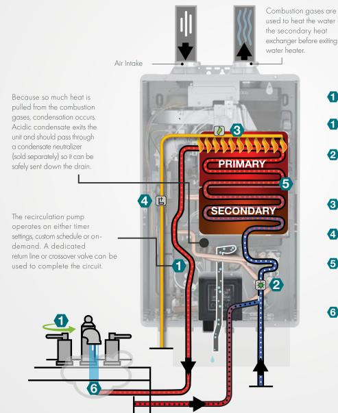
used to heat the water in the secondary heat exchanger before exiting the
