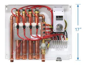
Units shall have enameled steel rated cover. Element shall be standard Emerson (or equal manufacturer) copper heating elements with threaded brass top. Unit shall have a replaceable mesh filter in the inlet. Heater shall be fitted with 1/2" plumbing connections for easy flex hose connection to eliminate need for soldering.
