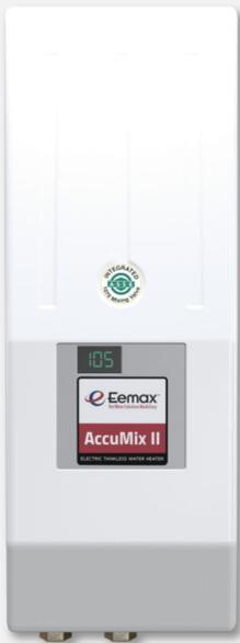
In order to meet the provisions of UPC 407.3, Eemax has added an ASSE 1070 code-compliant mechanical mixing valve to the AccuMix II Series of tankless electric water heaters. AccuMix II heaters feature an internally calibrated mixing valve and circuit board which work together to limit the hot or tempered water delivered at the faucet. With AccuMix II, the temperature of the heater is factory-set to 105 °F for handwashing applications.
