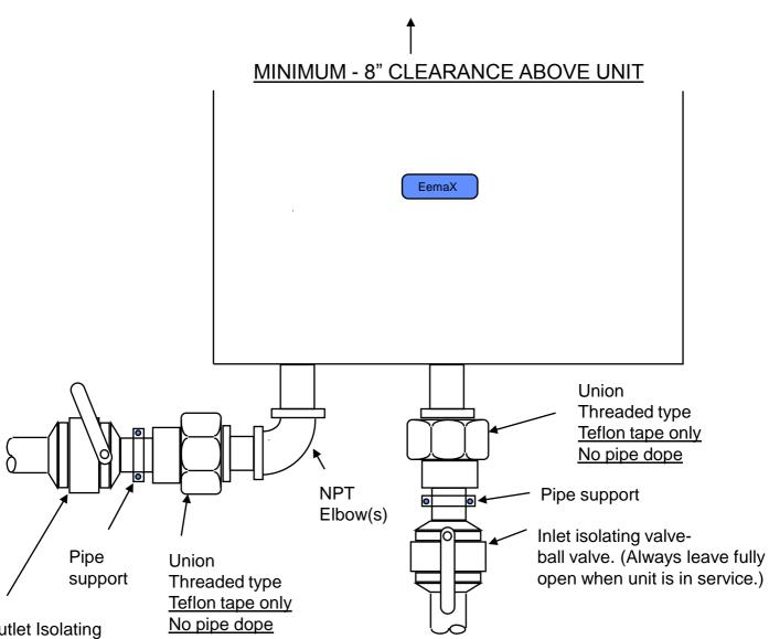
Outlet Isolating Ball Valve (throttle open just enough to obtain adequate flow of hot water)
