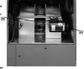
scroll provide quiet and efficient airflow. The blower sheave is secured by an "H" bushing which firmly secures the pulley to the blower shaft for years of trouble-free operation. The "H" bushing allows for easy removal of the blower pulley from the shaft, as opposed to the use of a set screw, which can score the shaft, creating burrs that make blower-pulley removal difficult.
