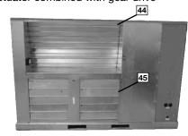
standard on all economizers. Power Exhaust is easily field installed. The power exhaust is housed in the barometric relief opening and is easily slipped in with a plugin assembly. The wire harness to the economizer also has accommodations for a smoke detector.
