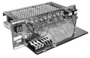
Power hook-up in the field is easy with single-point wiring to a terminal block (28) and a polarized plug for the low-voltage connection (29). The electric furnace comes with fuses for the unit (30) and for the electric furnace (31), and is UL certified (32). The electric heating elements are of a wound-wire construction (33) and isolated with ceramic bushings. The limit switch (34) protects the design from over-temperature conditions.
