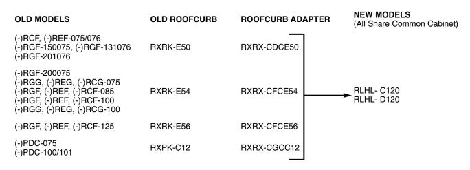
NOTE: Ductwork modifications may be necessary if the capacity and/or indoor airflow rate of replacement unit is not equivalent to that of the unit being replaced. RLHL- C120 or RLHL- D120 fits on the same curb as the RLKB- A090, A102, A120, A150, A181, RLMB- A090, A102, A120, A150, RLNB- A090, A102, A120
