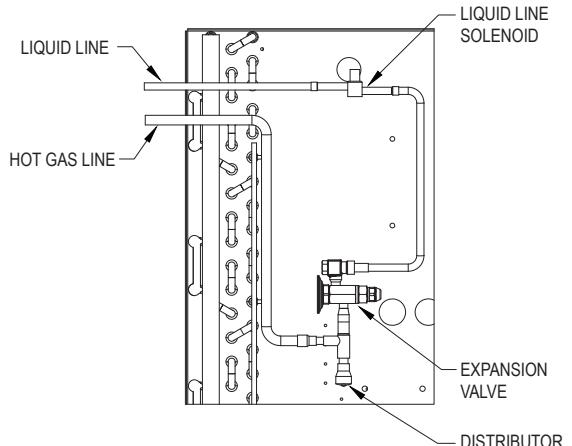
\* Each asterisk represents a variable character based on defrost and voltage ordered. Hot Gas 3-Pipe Version (H - Hot Gas Defrost 3-Pipe with Electric Drain Pan Heater, K - Hot Gas Defrost 3-Pipe with Hot Gas Drain Pan). See page 4 for nomenclature.
