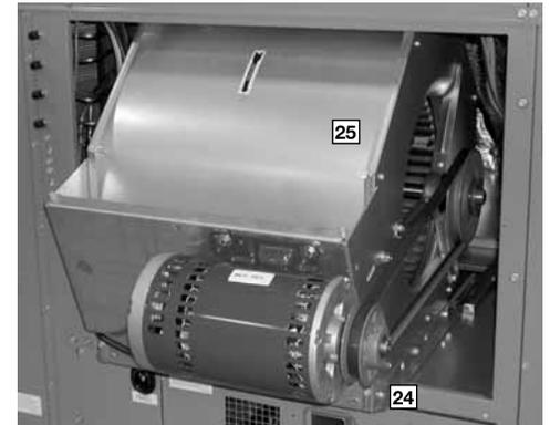
provide quiet and efficient airflow. The blower sheave is secured by an "H" bushing which firmly secures the pulley to the blower shaft for years of trouble-free operation. The "H" bushing allows for easy removal of the blower pulley from the shaft, as opposed to the use of a set screw, which can score the shaft, creating burrs that make blower-pulley removal difficult.
