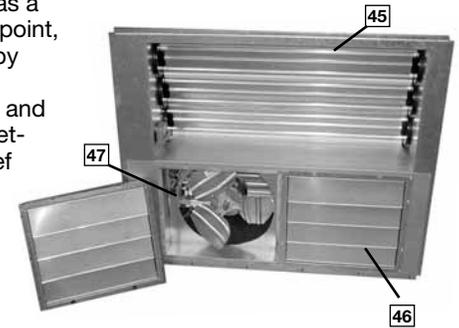
Power Exhaust (47) is easily field installed. The power exhaust is housed in the barometric relief opening and is easily slipped in with a plug-in assembly. The wire harness to the economizer also has accommodations for a smoke detector.
